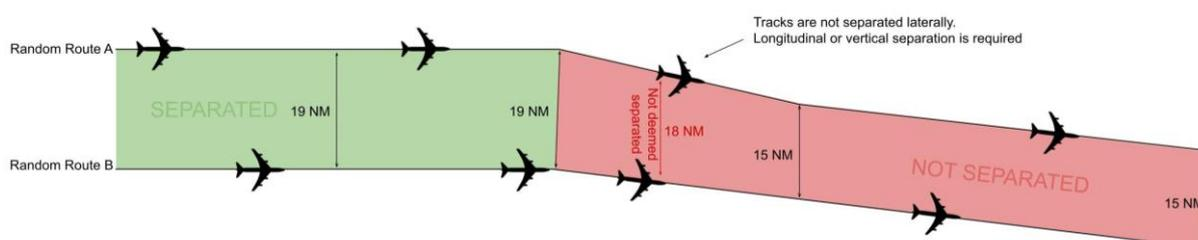
In Figure 2, aircraft A and B are laterally separated for the first portion of their route (green), however lateral separation does not exist once aircraft A's track deviates south. As soon as the first aircraft reaches the route portion that is no longer laterally separated, separation is lost. Therefore, another form of separation must be in place and separation ensured before this point is reached by either aircraft.
